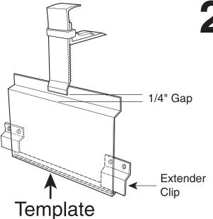
Once Deck Brackets are assembled starting at corners, set Template under Fascia Holder allowing 1/4" gap between bottom of Fascia Holder and Extender.
