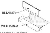
STEP 4: Installing Formed Retainer
