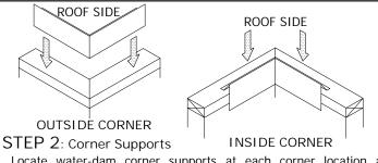
Locate water-dam corner supports at each corner location and fasten in place using 1-1/2" ss ring shank nails provided.
