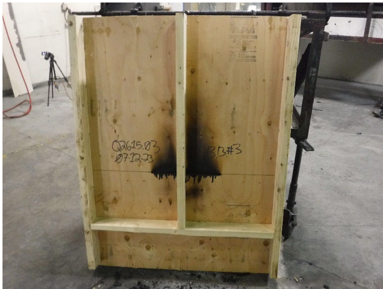
Photo No. 18 TEST #3 Underdeck Post Test
