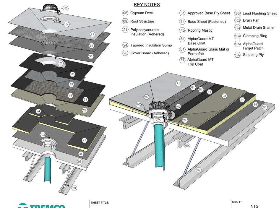
AlphaGuard® MT Plus Roof Drain Detail, Gypsum Deck
