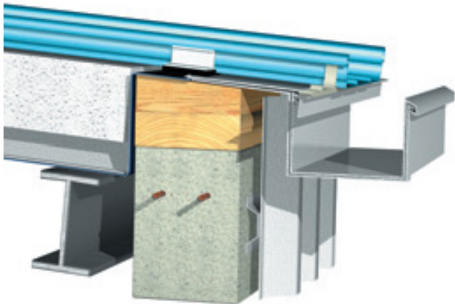
A = possible movement 0.4" / 10' (1.0 mm/m) TremLock K-Zip sheet
