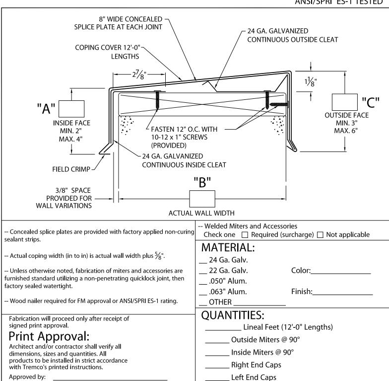
Date: FOR NON-90° MITERS SEE PRINT APPROVAL #60011-29182 PROJECT: TREMCO ROOFING AND BUILDING MAINTENANCE 3735 GREEN RD; BEACHWOOD, OH 44122 ARCHITECT: PHONE: 262-953-2666 **ROOFING CONTRACTOR:** EDGESYSTEMS@TREMCOINC.COM REPRESENTATIVE/DISTRIBUTOR: WWW.TREMCOROOFING.COM DATE: 07/19/18 SHT.# OF DRN BY: JJC
